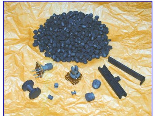
FSCP materials in injection moulding granules with moulded parts
